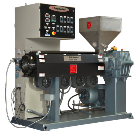
3 1/2-inch 24:1 Super Blue® extruder with discrete controls
