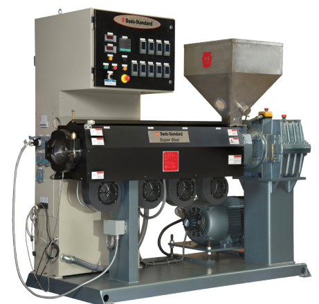
3 1/2-inch 24:1 Super Blue® extruder with discrete controls
