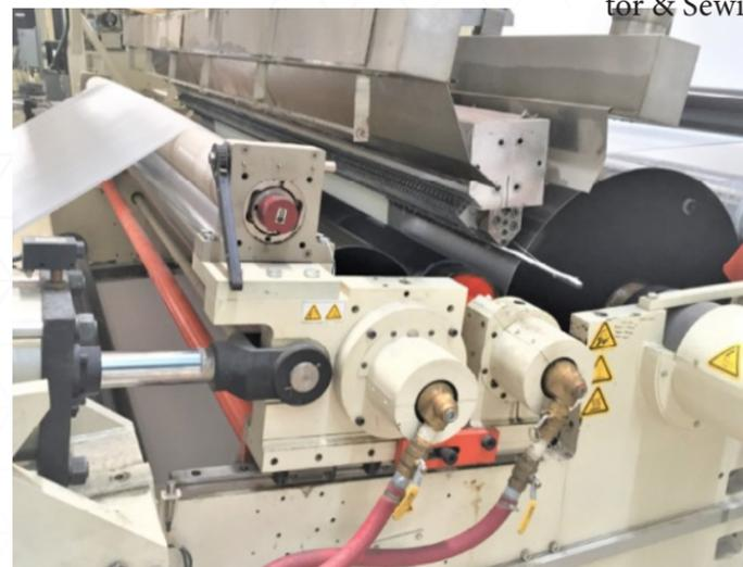
Unwind Unit with Accumulator & Sewing Machine
