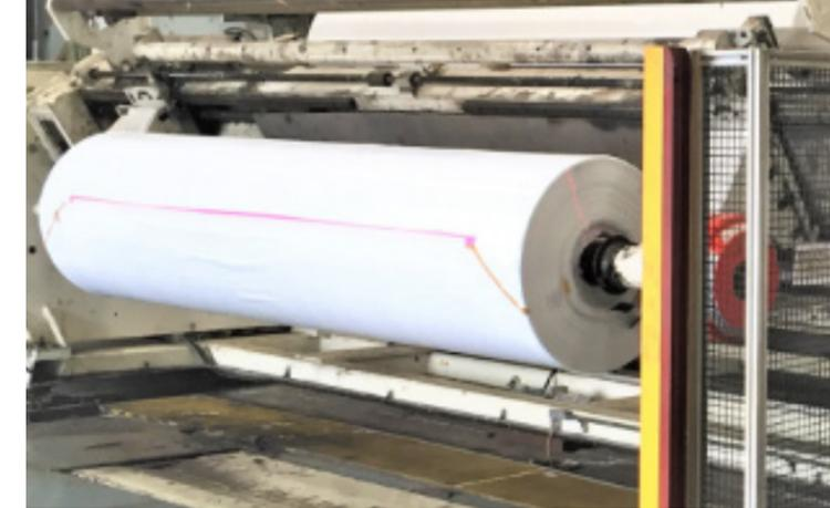
2-Position Turret Unwind Unit with Automatic Splicing
