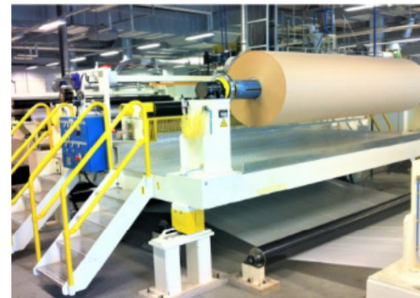
2-Position Fixed Auxiliary Unwind Unit
