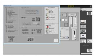
Davis-Standard's EPIC IV® integrates a high performance HMI experience with supervisory control for complex systems. With Windows®-based plant management and extensive process control capabilities, the EPIC IV can be customized for any extrusion or converting application. Supervisory features include alarm and event logging, customized real-time reports, SQC, historical trending, data collection, maintenance/troubleshooting help files, calibration, tuning, and more.
