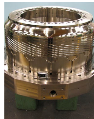
2" (50 mm) to 12" (300 mm) 5, 7 and 9-Layer coex stationary dies
