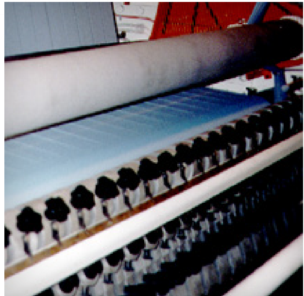
Davis-Standard's embossed film lines can in-line slit down to 2.5" (64mm) without bleed trim
