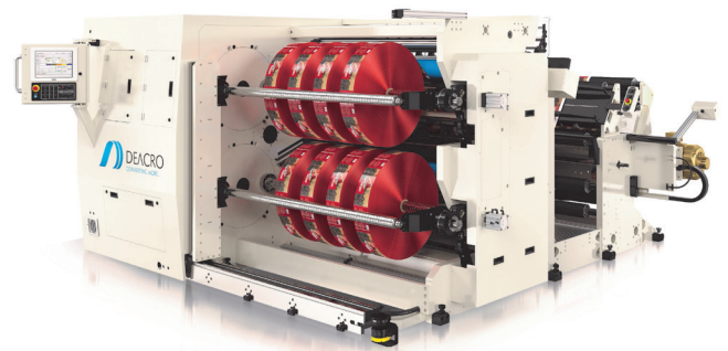
Pictured is the T800 turret slitter, which features an automated rewind and the ability to accommodate large OD rewrites.
