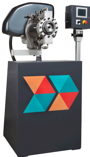
The Model 3000A features a proprietary automatic, servo driven concentricity adjustment system for improved processing.
